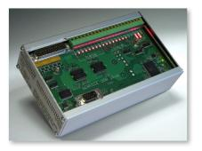
In general the interface is meant to be fixed by a metal angle (not supplied) in the back of a 19" rack. The USB interface can be disassembled for hole drilling. These holes can then be used for fixing.
