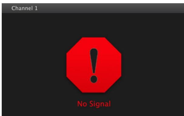
In the event of a signal loss or inconsistency, **Just In Multi** will display a “**No Signal**” alert to the user and stop the current recording in order to safeguard the recorded clip. Once the signal is back the user can restart the recording.
